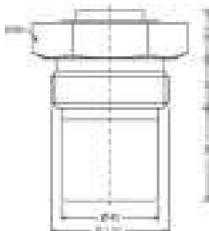
Type 5 – Thread ISO 228-1 – G 1 "A, front-flush
